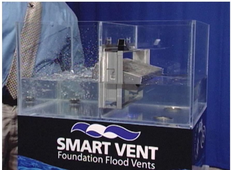
**Smart Vent's traveling tank illustrates how buoyancy of the stainless steel plate opens the vent automatically. Full demonstrations (live and on YouTube) show the plate switching directions when water begins flowing out of the structure as exterior floodwaters recede.**
