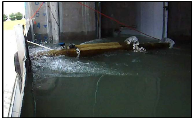
Log impact testing performed at ILC Test Facility
