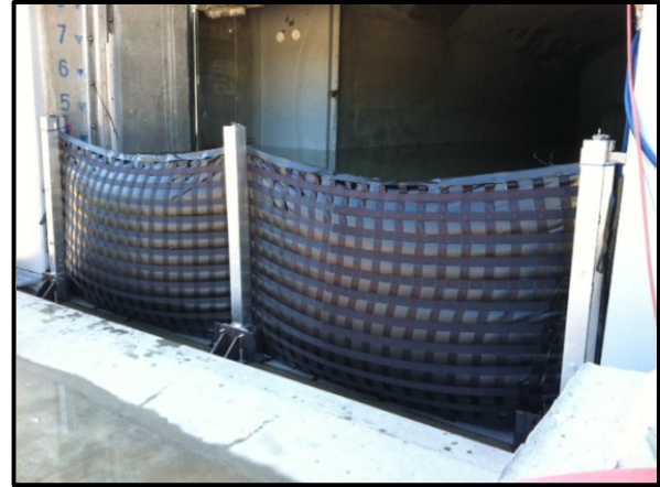
4' Tall x 16' Wide Flex-Wall™ tested at 3' of water
