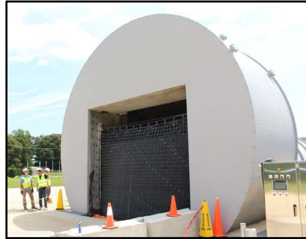
12' Tall x 16' Wide Flex-Wall™ tested at 10' of water
